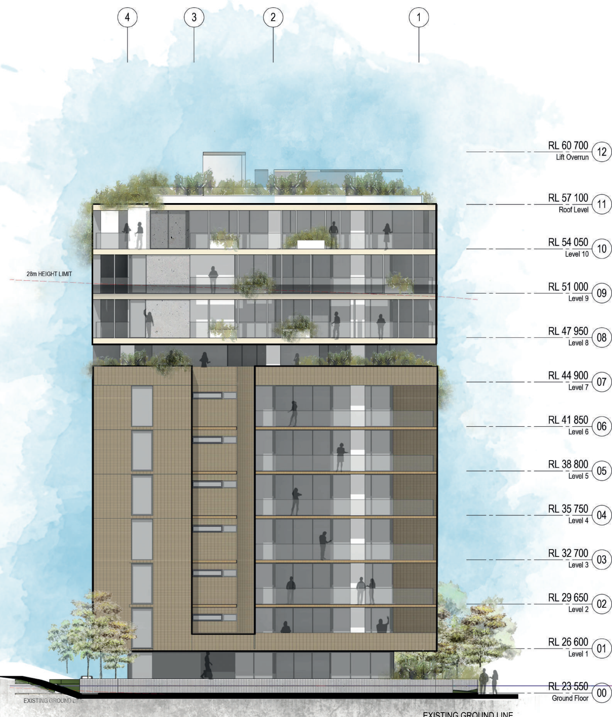
2 BUILDING B - EAST ELEVATION
